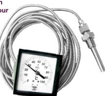
HAWK Industrial dial thermometers are designed to measure and indicate the temperature of a specific applications and conditions which are available in three actuation fills including liquid, mercury and gas. The dial thermometer can either be a directly local reading at the point of measurement or a remote reading by using a desired length of capillary tube. Model DTS is a remote design with a U-clamp for flushing mounting.
