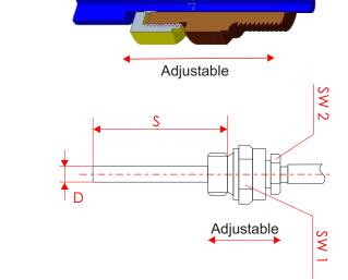
The sliding type allows to adjust the variable inserted
