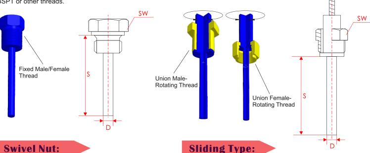
The swivel connector is a double male adapter. It allows you to move around to turn the position of the gauge face.
