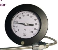
HAWK Industrial dial thermometers are designed to measure and indicate the temperature of a specific applications and conditions which are available in three actuation fills including liquid, mercury and gas. The dial thermometer can either be a directly local reading at the point of measurement or a remote reading by using a desired length of capillary tube. Model DBP is a hinged front remote design for flush mounting.
